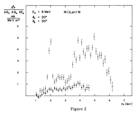
Differential cross sections for breakup leading to the ground states (○) and first-excited states (●) of the Ni isotopes.
