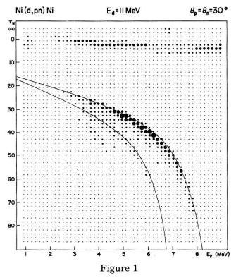
A two-dimensional plot of coincident events. The diameter of the points increases as a function of the intensity. Events from  $(d, d'\gamma)$  reactions are also present.
