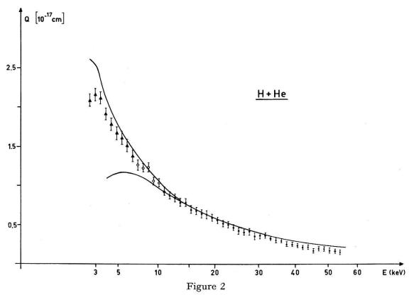
Total cross section for excitation of Lyman-radiation in H-He collisions. Full circles refer to hydrogen, triangles to deuterium data. Open circles represent the average of hydrogen and deuterium data. The upper solid line indicates the uncorrected values. The lower line is the distortion approximation. The energy scale has to be multiplied by two for deuterium.
