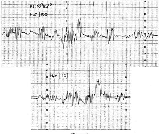
Figure 4 Spectres E.P.R., KI (Eu²+),  $H_0$   $\parallel$  [100] et  $H_0$   $\parallel$  [110]
