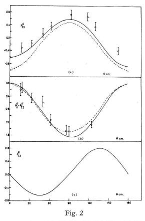
The polarization efficiency parameters, (a)  $P_{33}^d(\theta)$ , (b)  $P_{11}^d(\theta) - P_{22}^d(\theta)$ , (c)  $P_{13}^d(\theta)$ , for the reaction d+t at  $E_d=500$  keV. The dashed curve corresponds to s-wave resonance only.
