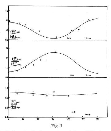
Polarized angular distributions for the d+t reaction at  $E_d=500$  keV, associated with deuteron polarization, (a)  $P_{33}=-0.28$ , (b)  $P_{33}=+0.14$  and  $P_{11}-P_{22}=-0.42$ , (c)  $P_{33}=+0.14$  and  $P_{11}-P_{22}=+0.42$ .
