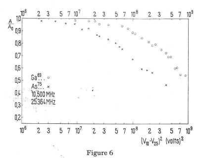
Saturation curves for Ga<sup>69</sup> and As<sup>75</sup> vs. the product of the squared voltages applied to the 10 MHz and 25 MHz transducers.
