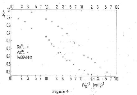
Saturation curves for Ga<sup>69</sup> and As<sup>75</sup> vs. the squared voltage applied at 14.864 MHz to a 15 MHz transducer. Conditions are maintained so that a given voltage applied to the transducer produces the same phonon energy density in the crystal for the saturation of both nuclei.
