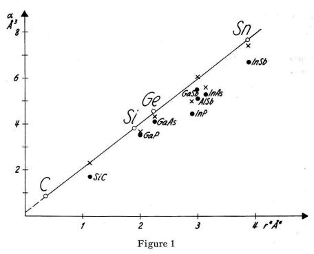
$\alpha$  calculated using (2) and plotted according to Kirkwood 9).  $\circ$  elements,  $\bullet$  compounds, where  $\frac{1}{2}(r_i^4 + r_k^4)$  is used instead of  $r_i \times \text{calculated}$  with formula (9), and with the slope K of the straight line for the elements
