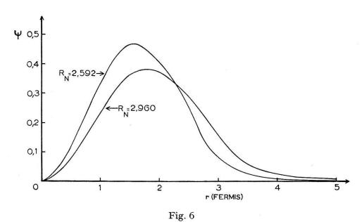
Bound state wave functions for the DWBA calculations with  $R_N = 2,592$  and 2,960 Fermis for the doublet state (5,20/5,25 MeV) of  $O^{15}$ .
