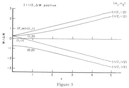
Energy level diagram for hydrogen in a magnetic field H, obtained from the Breit-Rabi equation:
