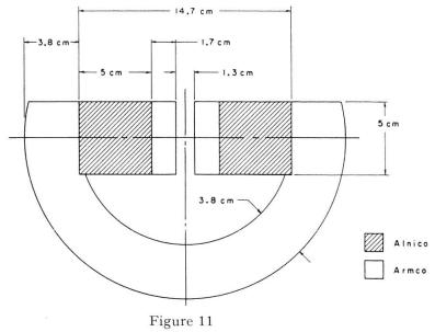
Cross section of homogeneous C-magnet, complete view
