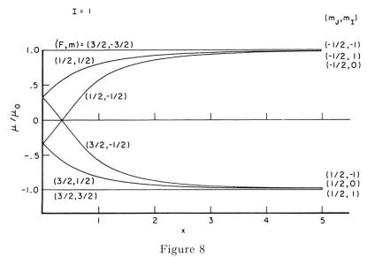
The magnetic moments of the magnetic sublevels of the hfs states of deuterium with J=1/2 and I=1 as a function of magnetic field H, obtained from the equations given in the caption to figure 6. Further description is the same as for figure 6
