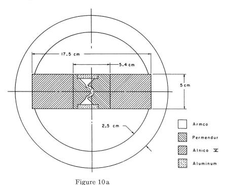
Cross section of iron deflecting magnet, complete view.
