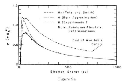
Ionization cross sections for atomic and molecular hydrogen as a function of electron bombarding energy. The solid (——) and dot-dash (———) curves refer to the process:  $e^- + H \rightarrow 2e^- + H^+$ . The dashed (———) curve refers to the process:
