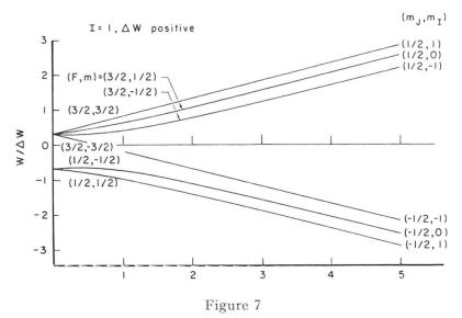
Energy level diagram for deuterium in a magnetic field H, obtained from the Breit-Rabi equation as given in caption to figure 5. For deuterium, J=1/2, I=1,  $\Delta \nu=327.38~Mc/s$ ,  $g_J=2.002$ , and  $g_I=-0.00047$ . Further description is the same as for figure 5
