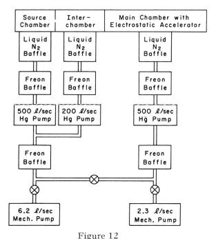
Schematic diagram of vacuum system
