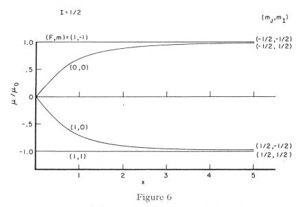
The magnetic moments of the magnetic sublevels of the hfs states of hydrogen with J=1/2 and I=1/2 as a function of magnetic field H, obtained from the equation:
