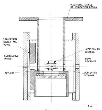
Figure 3 Ionization compartment
