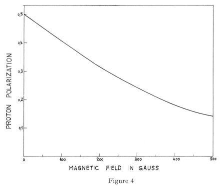
Proton polarization as function of field strength
