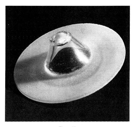
Figure 10 The collimator mounted on a 2 inch glass flange
