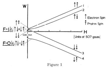
Energy levels of the hydrogen atom in a magnetic field
