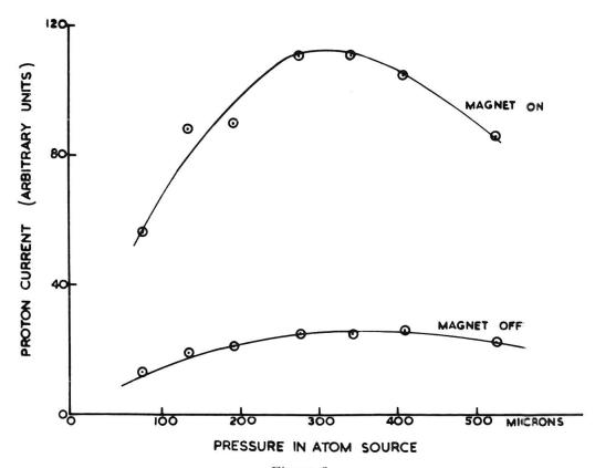
$Figure \ 5 \\ Proton \ currents-magnet \ on \ and \ off$
