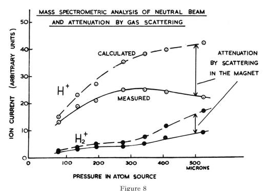
Mass spectrometric analysis of neutral beam and attenuation by gas scattering
