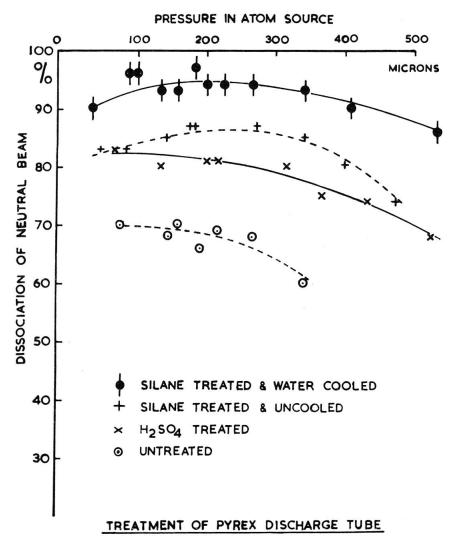
$Figure \ 12 \\$  Dissociation of neutral beam for different treatments of discharge tube
