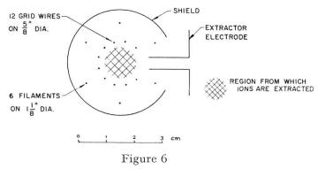
Cross section of the electron bombarder ionizer
