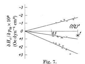
Calculated  $(\partial H_c/\partial p_\Theta)$  for Thallium specimens V—Tl—1  $\triangle$  V—Tl—3  $\nabla$  V—Tl—4 Hattons value at low pressures.
