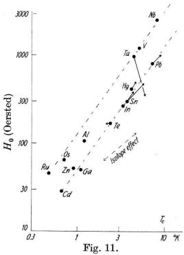
Effect of volume on  $T_c$  and  $H_0$ . The arrows indicate the direction and relative magnitude of motion in diagram resulting from increase in volume.
