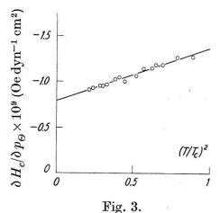
Calculated  $(\partial H_c/\partial p_{\Theta})$  for V—Sn—3.
