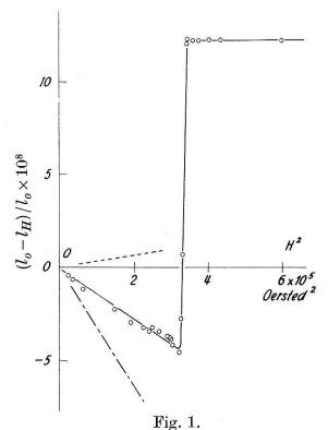
Change in length of lead rod V—Pb—4 at  $3\cdot 93^0$  K.  $(l_0-l_H)/l_0$  plotted against H<sup>2</sup>. Theoretical magnetostriction for infinite cylinder: ——— and for sphere: —————
