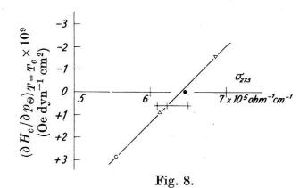
$(\partial H_c/\partial p_\Theta)$  at  $T=T_c$  as a function of conductivity  $\sigma_{273}$  at ice point for Thallium specimens. +++ indicates Hattons value plotted for different published values of conductivity.
