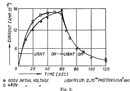
Rise and decay time of the primary photo current for two different initial voltages.
