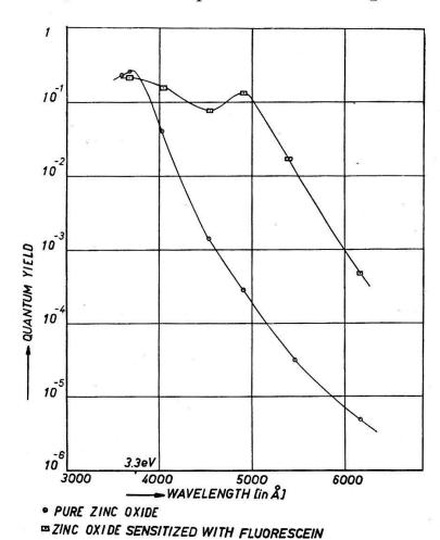
Fig. 4. Quantum yield in zinc oxide for different wavelengths.
