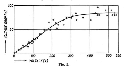
Voltage drop vs. initial voltage for a light flash of 7 x 10<sup>11</sup> photons/cm<sup>2</sup> of 3680 Å.
