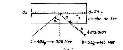
$$d\,N = \frac{N_0 \cdot d\,x \cdot \varOmega\left(x\right)}{2\,\pi} = (1 - x/L)\,d\,x\,N_0 \qquad N = N_0 \int\limits_0^d (1 - x/L)\,d\,x = N_0\,d\,(1 - d/2\,L)$$
