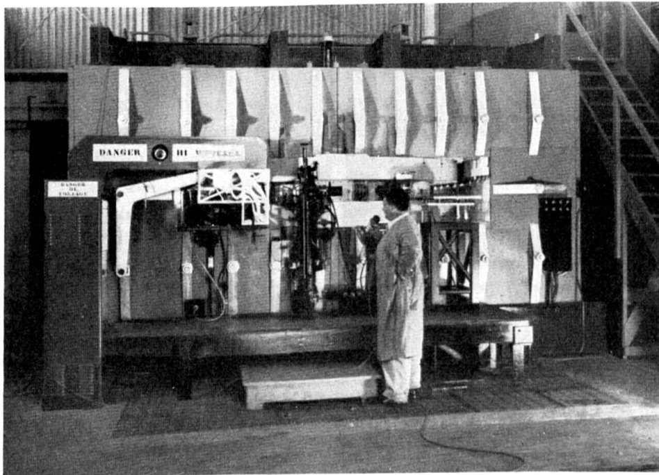
Fig. 12. Other side of synchrotron. The injector and its power supply are at the left, the x-ray beam emerges at the right, toward the observer.
