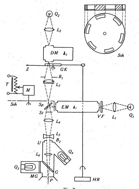
Fig. 3. Spektralflimmerphotometer.
