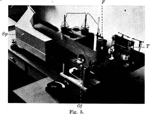
$F = {\bf Funke,} \quad Of = {\bf Ofen,} \quad Sp = {\bf Glasspektrograph,} \quad T = {\bf Transformator.}$
