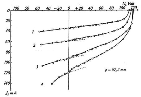
1) d = 2.2 mm 2) d = 1.8 mm 3) d = 1.4 mm 4) d = 1.0 mm Abstand Anode-Kathode 1.9 mm
