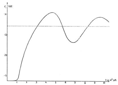
Fig. 5. ,,Tetroden-Multivibrator". (Vergl. Fig. 4).  $C_1 = 0.10~\mu\,F$ ,  $C_{12} = 0.005~\mu\,F$ ,  $r_1 = 10\,000~\Omega$ ,  $R_0 = 6\,800~\Omega$ ,  $E_0 = 150~\mathrm{V}$ ,  $e_0 = -27~\mathrm{V}$ ,  $\Delta~e_0 = 13~\mathrm{V}$ .
