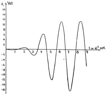
Fig. 7. Multivibrator (vergl. Fig. 6).  $C_1=C_1{'}=C_2{'}=0.10~\mu\,F,~C_2=0,~r_1=r_2=5000~\Omega,~R_1=R_2=10000~\Omega,~E_0=220~\mathrm{V},~\mathrm{R\"o}\mathrm{hre}$  Philips E.
