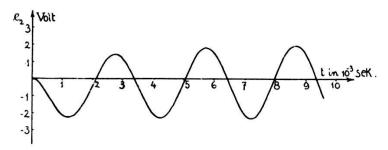
Fig. 8. Multivibrator (vergl. Fig. 6).  $C_1 = C_2 = C_1' = C_2' = 0.10 \ \mu F$ ,  $r_1 = r_2 = R_1 = R_2 = 6000 \ \Omega$ ,  $E_0 = 225 \ {\rm Volt}$ , Röhre Philips E.
