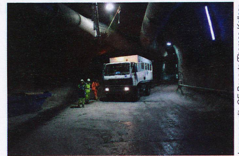
This Mercedes truck converted for passenger travel shuttles through a 3-kilometer-long tunnel (nearly 2 miles) built some 1,800 meters (5,900 feet) above sea level between the cable car and the power plant.
