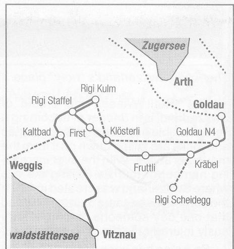
The picture shows the present 2 railway lines from Vitznau and Arth Goldau to Rigi-Kulm, the cable car from Weggis to Kaltbad and the proposed new cable car from Goldau to Rigi-Kulm via Klösterli.
