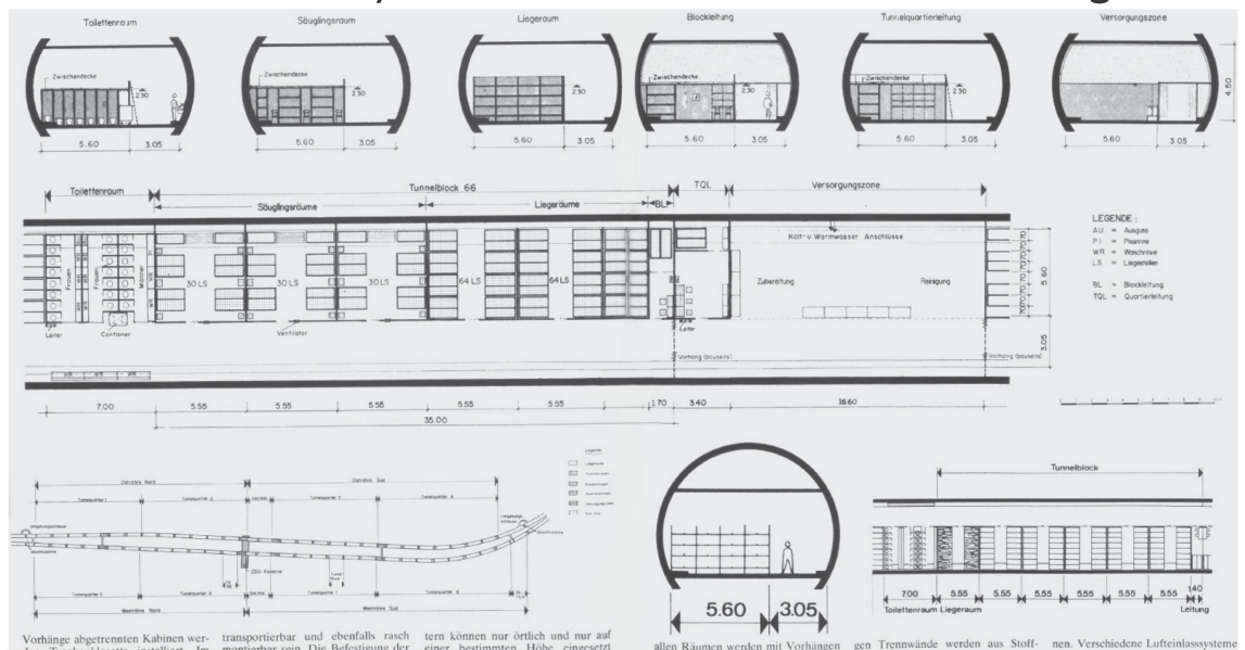
figs. 4 a–b Plan and section of the Sonnenberg highway tunnel when converted for occupancy (top) and section through the civil protection cavern (bottom). Source: M. Luchsinger, “Sonnenbergtunnel Luzern,” Zivilschutz 23, no. 9 (1976), 223–30, here 226–27.
