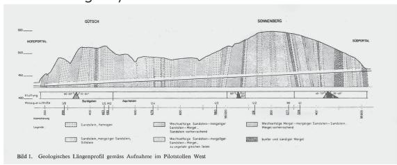
figs. 5 a-b Sections through the Sonnenberg funnel, showing the location within the mountain (top) and the cross-section of the tunnel (bottom). Source: E. Beusch and W. Studer, "Ausbruch und Verkleidung des Sonnenbergtunnels, Schweizerische Bauzeitung 90, no. 36 (Sep. 7, 1972), 853–57, here 854, 855.
