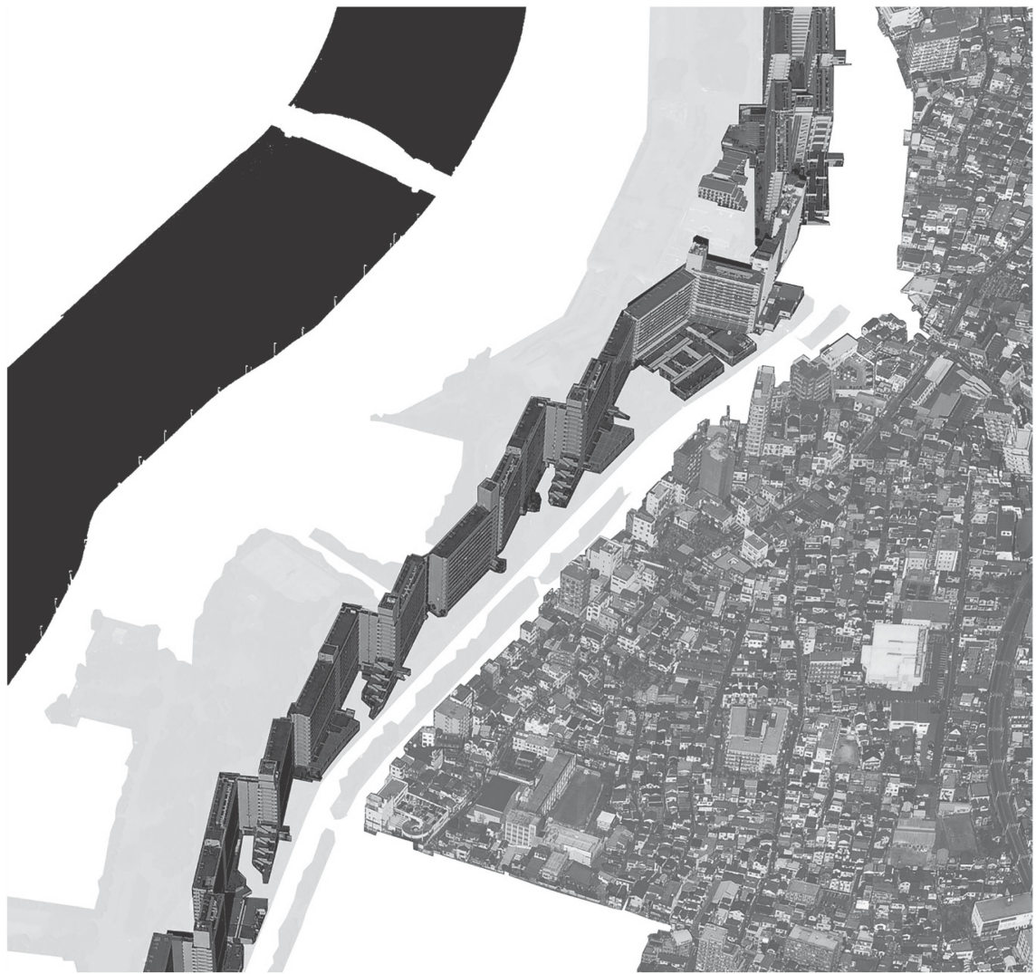
fig. 12 Urban paradigms: Shirahige Higashi. Complex of fifteen-story, interconnected housing units of reinforced concrete, creating a firebreak protecting the urban egress route beyond. Urban egress route follows the waterway (black), protected by firebreak buildings (darker tone) and fire-resistant planting (gray). Source: Max Ochel and Liam Ross.
