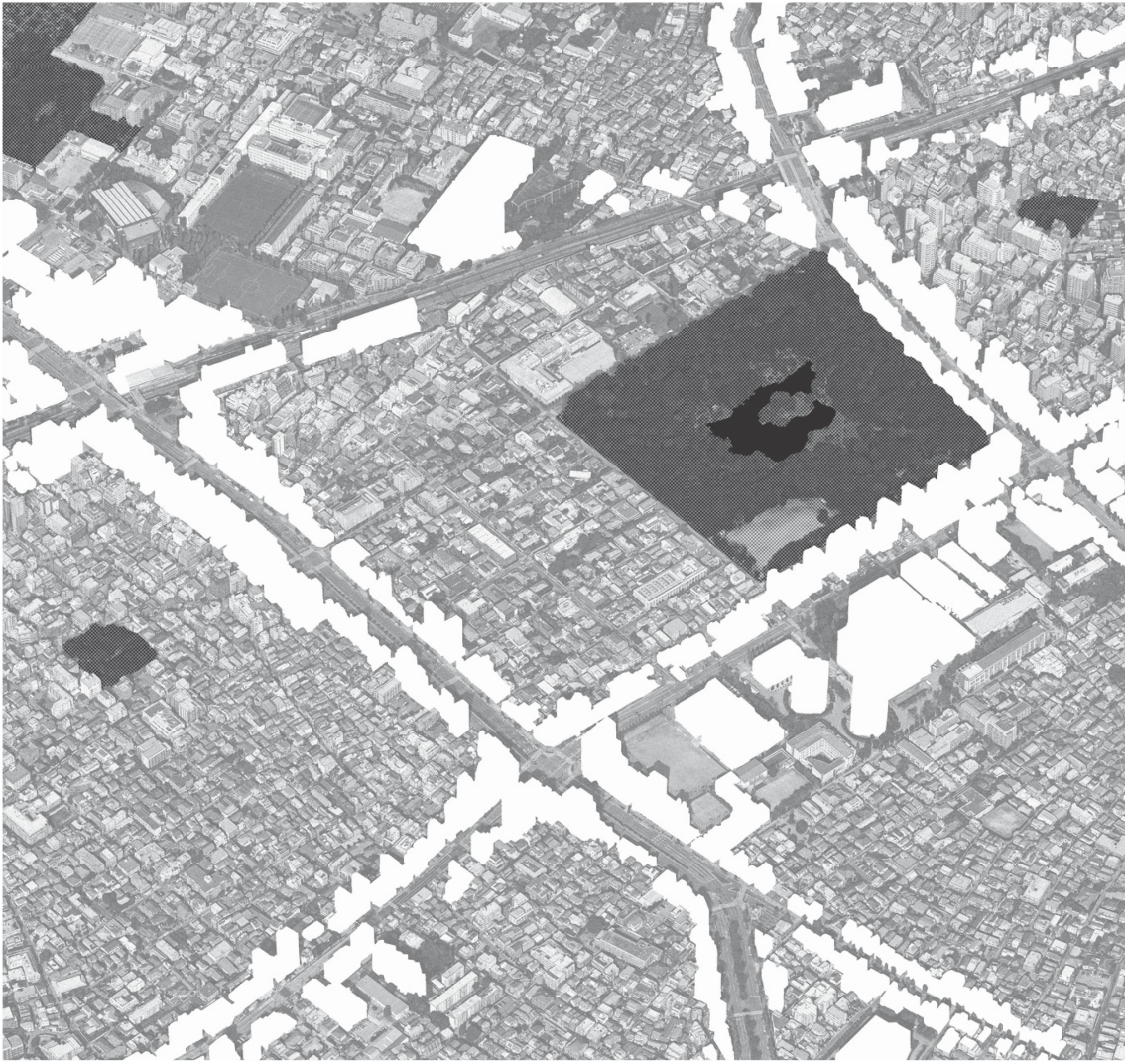
fig. 9 Urban paradigms: Sengoku Superblock. Example of a well-formed "hard shell / soft yolk" morphology. Note fire safety features of roads and waterways (black), firebreak buildings (white), and fire-resistant planting for urban muster zones (gray). Source: Max Ochel and Liam Ross.
