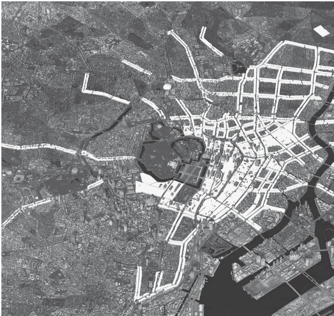
fig. 11 "Specters of Edo Castle." Swiss RE mapping of fire risk (darker tone) superimposed over City of Tokyo Fire Prevention Districts (white). After the Kanto earthquake, major routes were planned to be lined with firesafe construction, dividing the city into fire prevention "wards." White volume depicts designed height and depth of the urban fire wall. Note that contemporary fire risk reads as the inverse of the Kanto fire map; note also that areas of greatest fire risk are areas beyond the reach of planned fire-prevention construction. Source: Max Ochel and Liam Ross.
