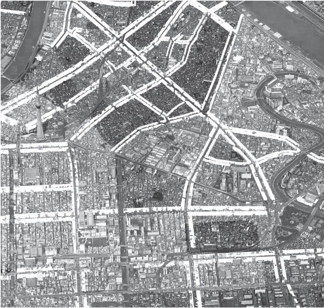
fig. 13 Incomplete castles: Sumida Ward. Contemporary fire risk in Sumida Ward (darker tone) superimposed with contemporary fire safety promotion zones (white). White volume depicts designed height and depth of urban fire wall; wherever this is visible, existing buildings fail to reach this height or depth. Note fire-risk patterns within dense low-rise areas and the incomplete state of firebreaks. Source: Max Ochel and Liam Ross.
