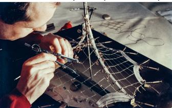
(as with a child's bubble f.4 Net model and wand) such soap films overall model on the measuring table, German Pavilion for take the shape of any the EXPO 1967 in closed, bent-wire form briefly dipped into then removed from them. 14 If 14 Cf. Daniela Fabricius, the bent-wire form describes a so-called space in Sonja Hildebrand curve then the soap film likewise constitutes a
