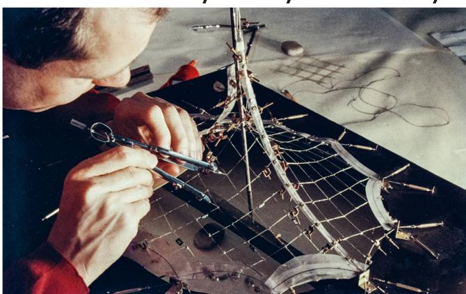
three-dimensional arcuate surface. In the course of countless experiments, Otto observed that a membrane of this sort is primarily defined by its contours, which is to say, its highest and lowest points; and also that it has specific geometric and physical properties. The surface tension in a soap film is identical at all
