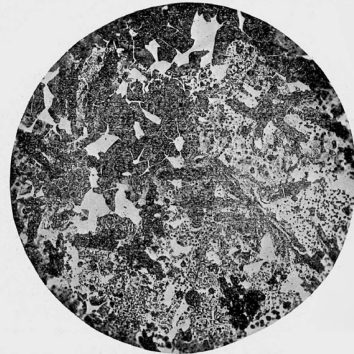
FIG. 2.—Advanced stage of weathering, Class I. Mag. \times 3 .
