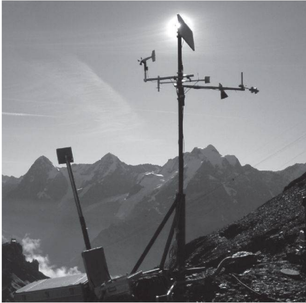
Fig. 2: (left) Meteo station, permafrost borehole and A-ERT installation at the northern slope of Schilthorn, Berner Oberland (2900 m a.s.l.). (right) Monthly specific resistivity values from the inversion results of continuous ERT measurements.
