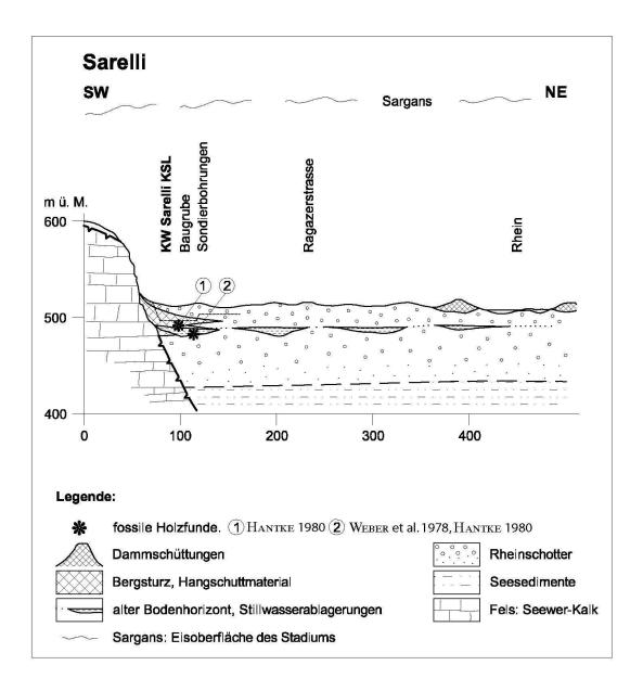
Fig. 2: Geologisches Querprofil: Sarelli (759'800/205'030) Geological cross-section: Sarelli (759'800/205'030) Coupe géologique: Sarelli (759'800/205'030) Graphik: Büro Dr. Max Kobel, Sargans
