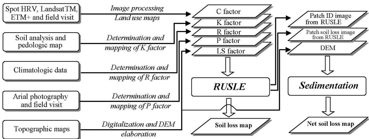
Fig. 2: Schematic presentation of the methodology
