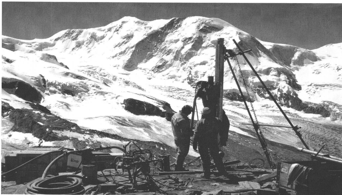
Photo 1: 100 m-deep borehole as part of the EU project PACE (Permafrost and Climate in Europe) on top of the Stockhorn (3420 m a.s.l.) at Zermatt, for long-term observation of the permafrost temperature in the rocks. In the background the frozen solid ice and cliff faces of the Lyskamm in the Monte Rosa Group.
