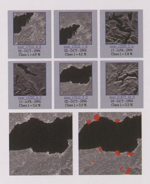
Fig. 8: Semantic CBIR on Synthetic Aperture Radar X-SAR SRL images of Switzerland Explanation: Top: Result of semantic query – discovering settlements. The images have been automatically analyzed at ingestion in the archive, and a catalog entry was created for all images containing built up areas. Bottom: Each image has attached to it the result of the classification. The regions marked in red correspond to villages and cities, thus the result of the search is a list of
