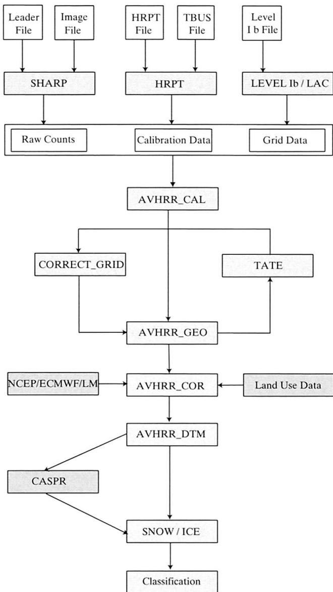
Fig. 2: NOAA-AVHRR processing chain designed for alpine studies with the modules calibration (AVHRR\_CAL), geocoding (AVHRR\_GEO), atmospheric and BRDF correction (AVHRR\_COR), orthorectification (AVHERR\_DTM), cloud masking (CASPR), snow classification (SNOW/ICE) and others
