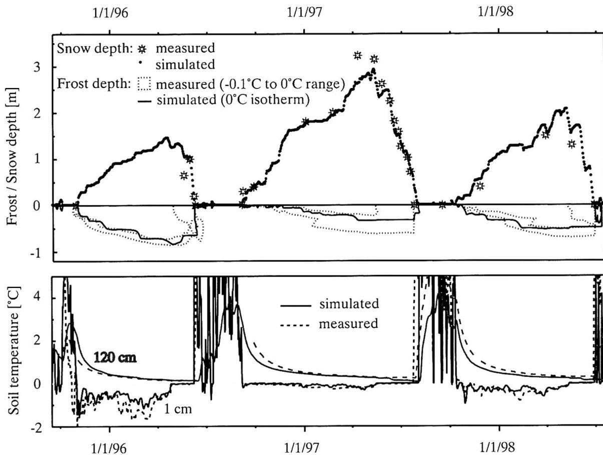
Fig. 4: Snow cover and ground thermal regime at a solifluction lobe at 2650 m a.s.l.: measurements and simulation results
