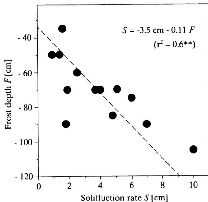
Fig. 6: Relation between annual frost depth (simulated) and solifluction rate (median of 7 marker measurements) between 1985 and 1998
