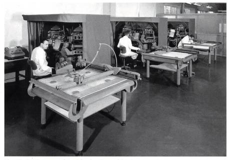
Fig. 10: A8 Autographs with plotting tables in operation.
