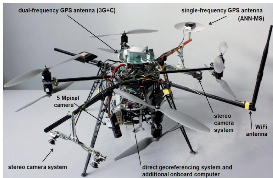
Fig. 2: The modified UAV with all sensor and processing components.
