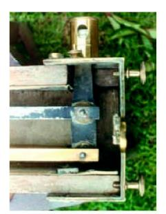
Fig. 4: The end of a Colby bar showing the two bars of different metal joined together in the arrangement to reduce the effect of temperature.
