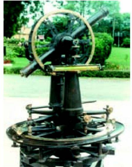
Fig. 6: 24 inch diameter theodolite used in India.
