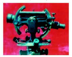
Fig. 5: Everest pattern theodolite designed by for use on revenue surveys.
