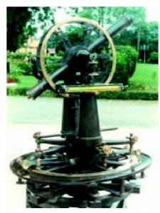
Fig. 6: 24 inch diameter theodolite used in India.
