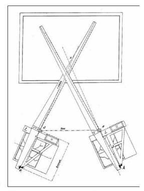
Abb. 3: Photogrammetrograph.
