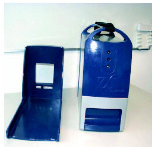
Fig. 4: flight data storage unit FDS.
