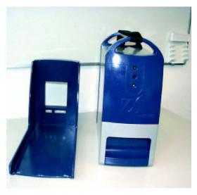
Fig. 4: flight data storage unit FDS.
