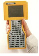
Trimble today introduced the TSCe™ Controller, the latest addition to the Trimble Toolbox™ of Integrated Surveying™ solutions. The TSCe is a powerful handheld data collector that uses sight, sound and touch to allow surveyors to conduct multiple tasks quickly and accurately.
