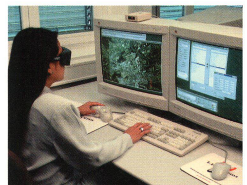
Abb. 2: Digitale Photogrammetrische Station.
