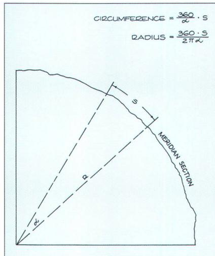
Fig. 2: Principle of determining size of earth as a sphere.
