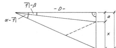
$$\begin{aligned} D &\hat{=} 1 \\ \alpha - \beta &\hat{=} \tan(\pi - \beta) = 0,235 \\ \beta &\hat{=} \tan(\alpha - \pi) = 0,675 \\ x &= \beta - a = 0,440 \hat{=} 400 \text{ m} \\ D &= \frac{400}{0,44} = \underline{\underline{909 \text{ m}}} \end{aligned}$$
