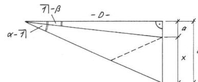
$$\begin{aligned} D &\hat{=} 1 \\ a &\hat{=} \tan(\pi - \beta) = 0,235 \\ b &\hat{=} \tan(\alpha - \pi) = 0,675 \\ x &= b - a = 0,440 \hat{=} 400 \text{ m} \\ D &= \frac{400}{0,44} = \underline{\underline{909 \text{ m}}} \end{aligned}$$
