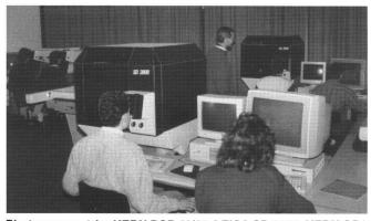
Photogrammetrie: KERN DSR 11/15, LEICA SD 2000, KERN GP1 Plotter.
