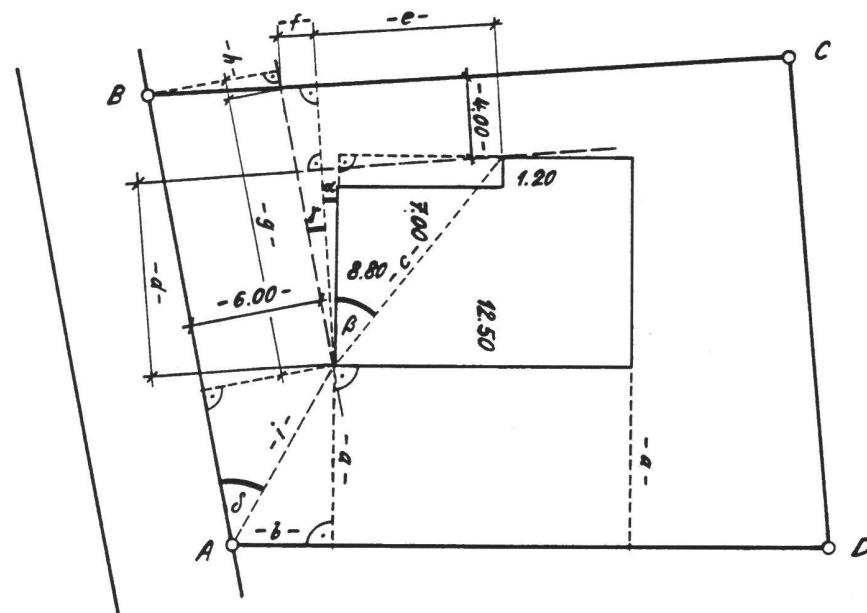
$$Az_A^B = 365.974^\circ \quad \overline{AB} = 20.220 \text{ m}$$
