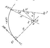
$NW = 350^{9}$   $Az K1 \rightarrow Z = 50^{9}$  YZ = 5000, XZ = 1200  $AZH \rightarrow Z = 150^{9}, \overline{HZ} = 565.685m$   $AZH \rightarrow J = 107.9167^{9}$   $\alpha = AZH \rightarrow Z - AZH \rightarrow J = 42.0833^{9}$   $\alpha = \overline{HZ} \cdot \sin \alpha = 347.297m$   $\sin \beta = \alpha : R, \beta = 22.5801^{9}$   $J = AZH \rightarrow J + \beta - AZK1 \rightarrow Z$   $J = 80.4968^{9}, \Delta K = R \cdot arc_{J}$   $\Delta K = 1264.441m$  KX = 2.264441Km
