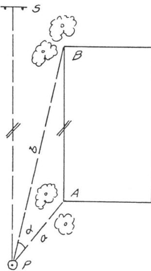
$$\begin{aligned} a &= 6.403 \text{ m} \\ b &= 17.464 \text{ m} \\ r &= 28.243 \text{ m} \end{aligned}$$
