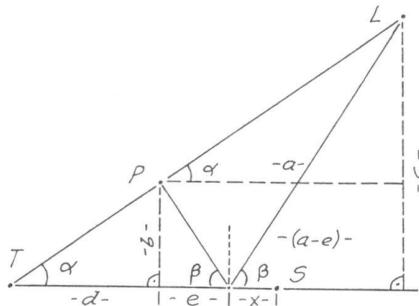
$$\begin{aligned}TP &= 10.817 \text{ m}, \gamma = 37.433^\circ \\PL &= 17.307 \text{ m}, TS = 13.100 \text{ m} \\a &= PL \cdot \cos \alpha = 14.400 \text{ m} \\b &= TP \cdot \sin \alpha = 6.000 \text{ m} \\c &= (TP+PL) \cdot \sin \gamma = 15.600 \text{ m} \\d &= TP \cdot \cos \gamma = 9.000 \text{ m} \\b : e &= c : (a-e) \\ce &= ab - be \\e(b+c) &= ab \\e &= ab : (b+c) = 4.000 \text{ m} \\x &= TS - (d+e) = 0.100 \text{ m}\end{aligned}$$
