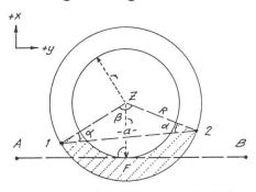
$Az 1 + 2 = 94.877^{9}, a = 12.541m$   $cos \varphi = 9/2 : R, \varphi = 29.323^{9}$   $Az 1 + Z = Az 1 + 2 - \varphi = 65.554^{9}$  yz = 9.000, Xz = r = 4.999m  $\beta = 200^{9} - 2 \varphi = 141.354^{9}$   $F = [(R^{2} - r^{2}) arc \beta] : 2$   $F = 26.66m^{2}$
