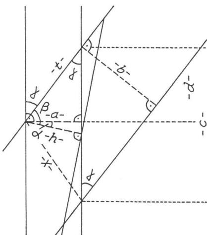
$$\begin{aligned} \cos \alpha &= a : h, \alpha = 12.565^\circ \\ \cos \beta &= h : t, \beta = 70.484^\circ \\ \gamma &= 100^\circ + \alpha - \beta = 42.081^\circ \\ c &= b : \sin \gamma = 13.429 \text{ m} \\ d &= a : \tan \gamma = 6.429 \text{ m} \\ x &= \sqrt{a^2 + (c-d)^2} = 8.602 \text{ m} \end{aligned}$$
