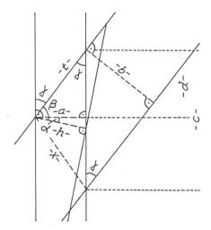
$cos \ \alpha = \alpha : h, \ \alpha = 12.565^{\circ}$   $cos \ \beta = h : t, \ \beta = 70.484^{\circ}$   $j = 100^{\circ} + \alpha - \beta = 42.081^{\circ}$  c = b : sin j = 13.429 m  $d = \alpha : tan j = 6.429 m$  $x = \sqrt{\alpha^2 + (c-d)^2} = 8.602 m$
