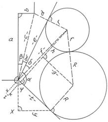
$c = \sqrt{a^2 + b^2} = 10.548m$   $tan \beta = b : a, \beta = 18.832^9$   $e = \sqrt{c^2 - d^2} = 10.051m$   $sin_f = d : c,_f = 19.623^9$   $f = \sqrt{e^2 + r^2} = 10.818m$   $tan \delta = r : e,_{\delta} = 24.1/2^9$   $y = 200^9 - (\alpha + \beta + f) = 37.795^9$   $h = f sin(\alpha - \delta) - R = 4.768m$   $i = f cos(\alpha - \delta) = 0.062m$   $g = \sqrt{(R + r)^2 - h^2} = 8.847m$  t = g + i = 8.909m x = t cos y = 7.385m y = t sin y = 4.984m
